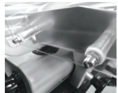
4. Screw on the two dome nuts.
